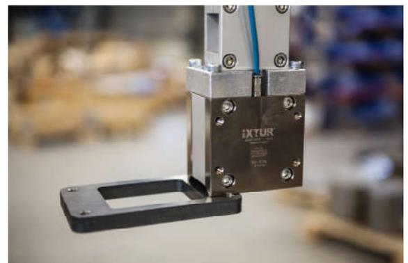
The magnets do not change their magnetic state in case of loss of compressed air.
